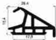
HL16 İZOLE KANAT FİTİLİ GENİŞ PK 15 KG/75 M ISOLATED SASH GASKET LARGE
