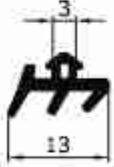
HL06 HİLAL YALITIMSIZ YATAK FİTİLİ S57 PK 15 KG / 294 M HİLAL GLASS GASKET S57
