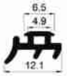
HL32 ECO CAM ALT FİTİLİ PK 15 KG/326 M ECO GLASS'S BOTTOM GASKET
