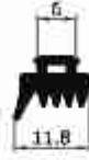
HL29 KASA FİTİLİ S57 (E84) PK 15 KG/200 M SAFETY GASKET S57 (E84)
